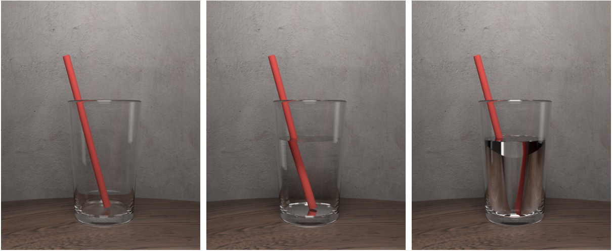
Figure 5.1: A sequence of side-view images depicting an empty glass with \eta = 1.5 (left), a glass containing water with \eta = 1.33 (middle) and a glass containing a liquid NIM with \eta = -1.33 (right).
