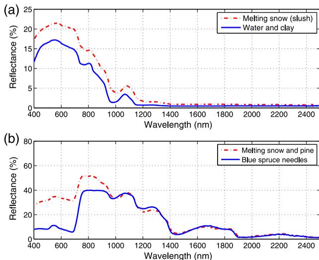
**Fig. 3** Reflectance spectra<sup>9</sup> for sample materials characterized by the presence of prominent features at the NIR wavelengths of interest. (a) Melting snow (slush) and water mixed with clay (1.67 g/L). (b) Melting snow mixed with forest vegetation (pinyon pine), and fresh blue spruce needles.
