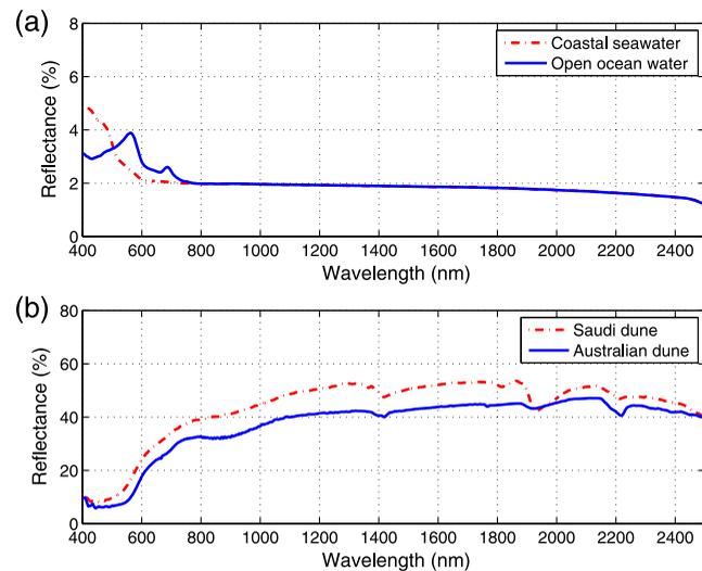
**Fig. 2** Reflectance spectra for sample materials characterized by the absence of prominent features at the near-infrared (NIR) wavelengths of interest. (a) Ocean water samples.<sup>9</sup> (b) Desert (dune) sand samples.<sup>10</sup>
