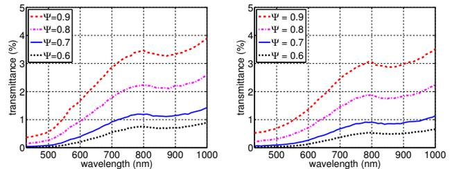
**Fig. 4.** Comparisons of modeled transmittance curves obtained for the selected Martian regolith samples, B (left) and D (right), considering distinct values for the average sphericity ( $\Psi$ ) of their grains and a thickness of 0.8 mm.
