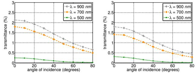
**Fig. 3.** Graphs depicting the angular dependence of modeled transmittance curves obtained for the selected Martian regolith samples, B (left) and D (right), considering three representative wavelengths ( $\lambda$ ) and a thickness of 0.8 mm.
