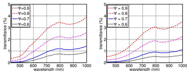
**Fig. 4.** Comparisons of modeled transmittance curves obtained for the selected Martian regolith samples, B (left) and D (right), considering distinct values for the average sphericity ( $\Psi$ ) of their grains and a thickness of 0.8 mm.
