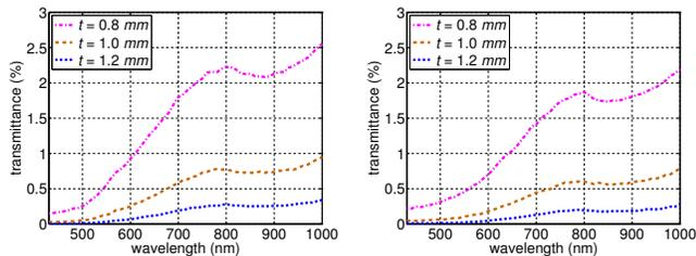
**Fig. 2.** Comparisons of modeled transmittance curves obtained for the selected Martian regolith samples, B (left) and D (right), considering distinct values for their thickness ( $t$ ).
